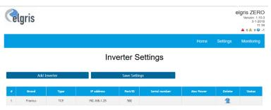
After selecting the brand of the inverter which needs to be controlled, the type of communication needs to be selected. Not all communication options are available for all inverters. Please refer to the inverter support list on the website <a href="https://www.elgrispower.com">www.elgrispower.com</a>
